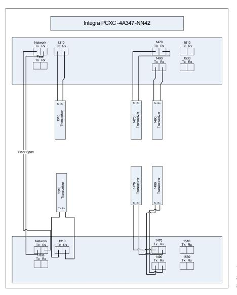
The Integra Optics passive CWDM units and transceivers supplied to our customer, showing room for additional expansion.
